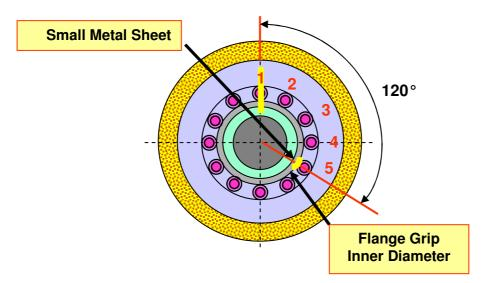
A second spindle rotation is conducted to the production RPM and a second vibration check is monitored. This process is repeated till the flange set is meeting the vibration goal. A normal acceptable vibration value is in the range of 0.02mm / sec<sup>2</sup> but this value may change per each application requirement.
