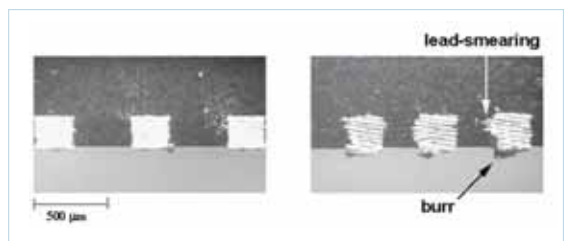
Figure 1: Micrographs of the cross sections of diced QFN samples demonstrating variations in cut quality. Left - cut quality within specifications; Right - large burrs and extensive smearing of leads
