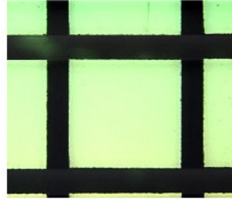
Borosilicate substrate diced at 1mm / sec
