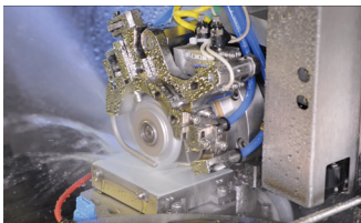
Blade preparations using automatic 75mm x 75mm dressing station
